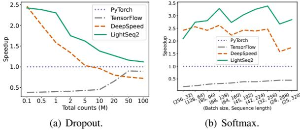
Fig. 17. Speedup for Dropout and Softmax operators.
