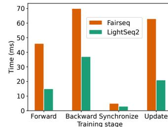
Fig. 3. Time cost for Fairseq and LightSeq2 based on WMT-14 English-German machine translation task, using Transformer-24e24d and 8 Tesla A100 GPUs.
