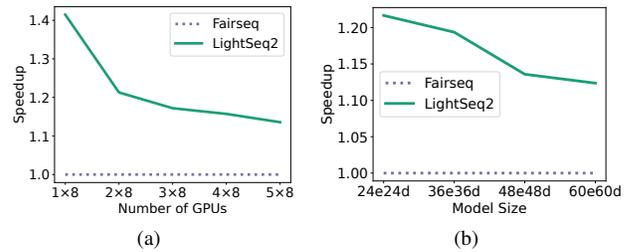
Fig. 22. Scalability of LightSeq2. (a) Speedup on different numbers of A100 GPUs for 48e48d model. Here  $5 \times 8$  represents five nodes with eight GPUs on each (40 GPUs in total). (b) Speedup for varying sizes of models on  $5 \times 8$  A100 GPUs. 60e60d has a total of 120 Transformer layers.
