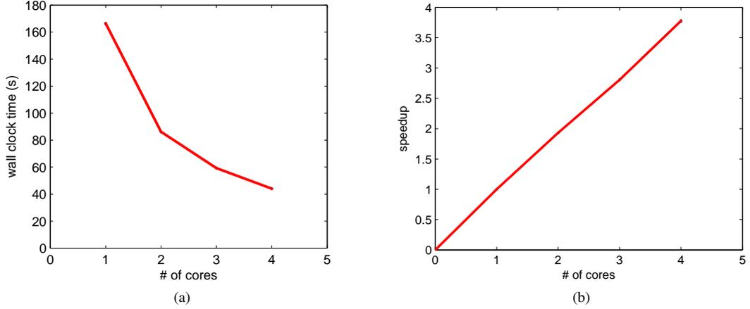
**Fig. 6** Performance of *Cut-And-Stitch* HMM on multi-core desktop, (a) running time versus number of cores  $k$ ; (b) speedup versus number of cores  $k$ .
