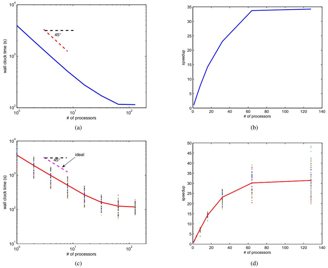
**Fig. 4** Performance of *Cut-And-Stitch* LDS on NCSA supercomputer, running on the 58 motions. The Sequential version is on one processor, identical to the EM algorithm. (a) Running time for a sample motion (subject 16 #22, walking, 307 frames) in log-log scales; (b) Speedup for walking motion(subject 16 #22) compared with the sequential algorithm; (c) Average running time (solid line) for all motions in log-log scales. (d) Average speedup for all motions, versus number of processors  $k$ .
