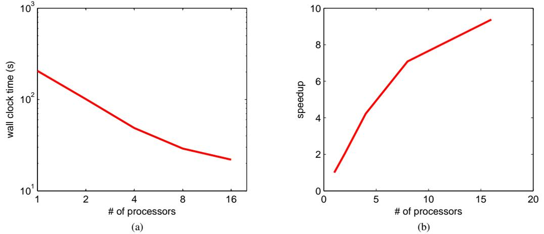
**Fig. 7** Performance of *Cut-And-Stitch* HMM on PSC supercomputer, (a) running time versus number of cores  $k$  in log-log scale; (b) speedup versus number of cores  $k$ .
