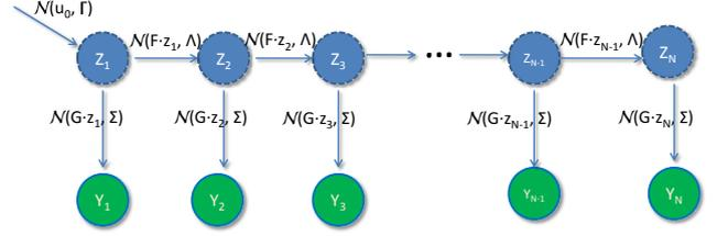
**Fig. 1** A Graphical Representation of the Linear Dynamical System:  $\mathbf{z}_1, \dots, \mathbf{z}_N$  indicate hidden variables;  $\mathbf{y}_1, \dots, \mathbf{y}_N$  indicate observation. Arrows indicate Linear Gaussian conditional probabilistic distributions.
