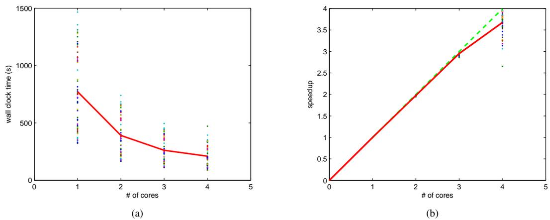
**Fig. 5** Performance of *Cut-And-Stitch* LDS on multi-core desktop, running on the 58 motions. The Sequential version is on one processor, identical to the EM algorithm. (a) running time for all motions; (b) average speedup for the 58 motions, versus number of cores  $k$ .
