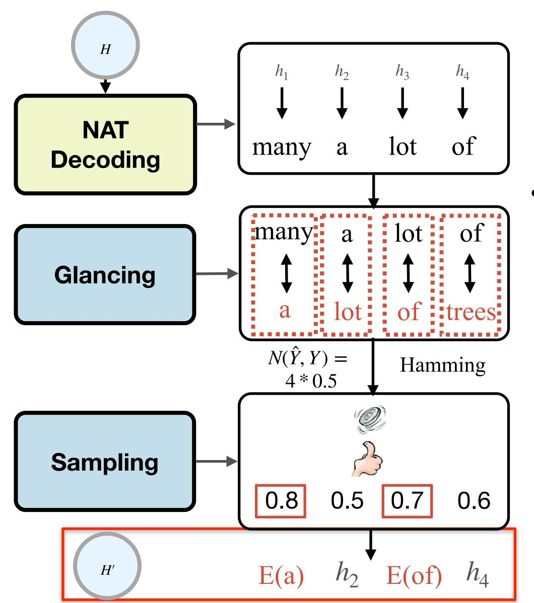
Replace the original decoder inputs with the embedding of sampled target words
